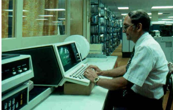
Figure 3.4. Univac 1108 mainframe console. Note 12” tape reels in background. Contents of about 6,000 such reels can now fit on a single 300GB 3.5” disk.
