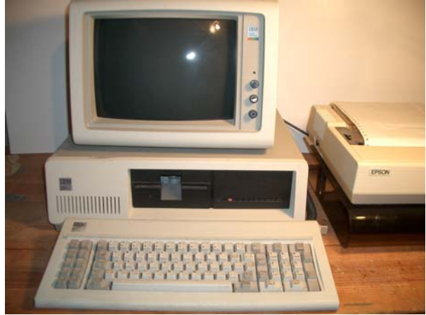
Figure 3.9. First IBM PC/XT and printer bought for departmental office in 1984 at a cost of $5700. (Photo by M. Zelkowitz)
