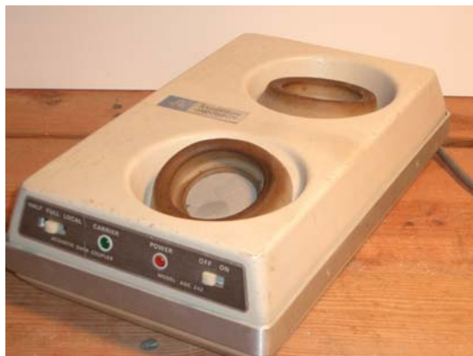
Figure 3.5. This 300 bps acoustic coupler modem was the main faculty device for connecting home terminals to the Univac 1108 mainframe in the 1970s. (Photo by M. Zelkowitz)
